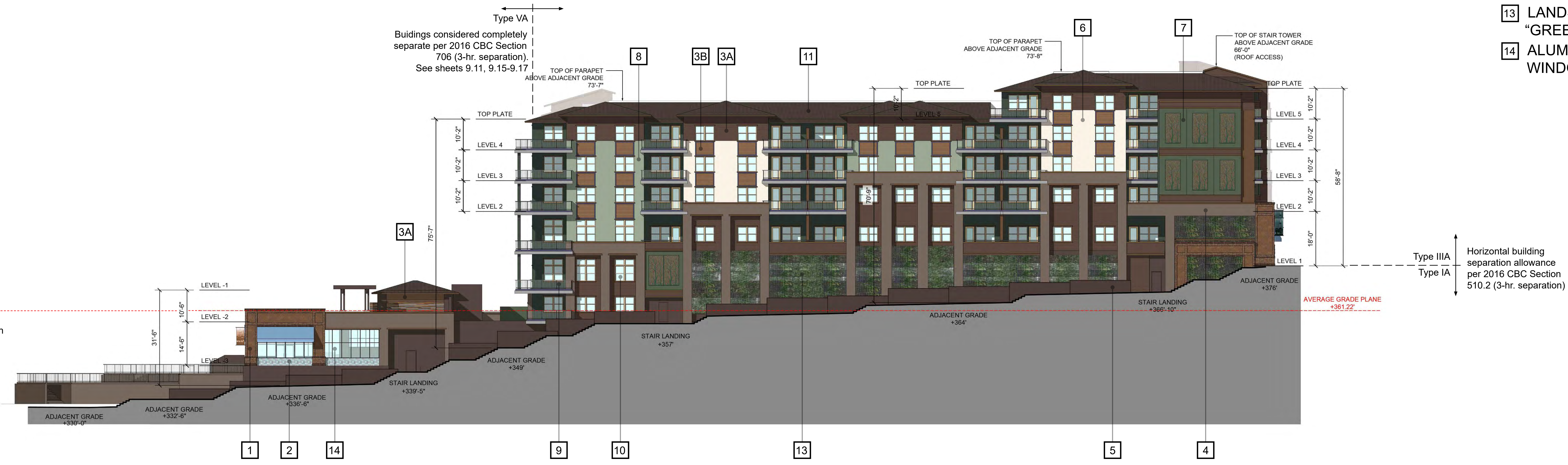
2. WEST STAIRWAY ELEVATION
